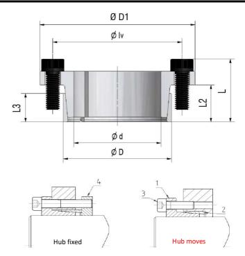
Ma: screw tightening torque Mt: transmissible torque (Fax=0) Fax: transmissible axial load (Mt=0)
