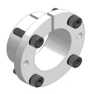
Low torque capacity Low contact pressures Self-locking & self-centering Axial fixation of hub during tightening: yes / no Max tolerances: shaft h8; hub bore H8 Shaft / hub bore surface finish:  $0.8 \le Ra \le 3.2 \ \mu m$
