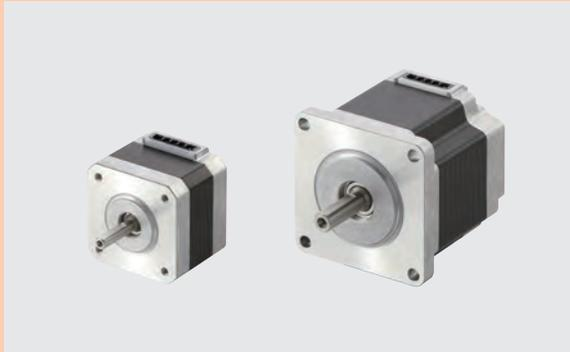
This is a high torque and low vibration stepper motor with a basic step angle of 0.72° (resolution of 500 steps per revolution). High positioning accuracy is possible through low vibration and reduced noise. (A separate dedicated driver is required to operate each motor.)
