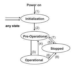
After Power On and initialization, the slaves are in the Pre-Operational state. The transition (2) is automatic. The system bus master (frequency inverter or PLC/PC) triggers the transition (3) to Operational state. The transitions are controlled via NMT telegrams.
