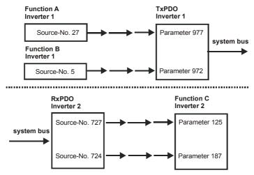
Example 2 displays the same situation as Example 1. But now, the functions A and B are in frequency inverter 1 and function C in frequency inverter 2. The connection is done via a TxPDO in frequency inverter 1 and a RxPDO in frequency inverter 2. Thus, the parameterization for this connection is:
