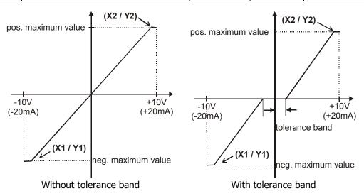
The *Minimum Frequency* **418** or the *Minimum reference percentage* **518** set in the factory extends the parameterized tolerance band to the hysteresis.
