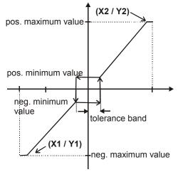
With tolerance band and minimum value
