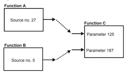
In example 1, the two inputs of function C are connected to the outputs of functions A and B. The parameterization for this connection is thus:
